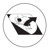
After the prompt, "Next, Separate One of the White Pads Completely from Blue Plastic Liner. Begin Peeling from the Tabbed Corner," with a firm, steady pull, carefully peel one pad away from the blue release liner.
