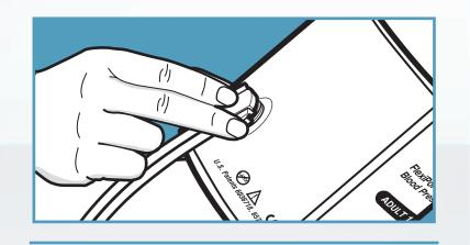
Snap the FlexiPort fitting, from the device directly into the cuff.
